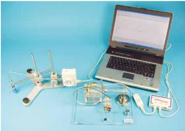
**10457 Motor Stirling II. Diagrama PV**
